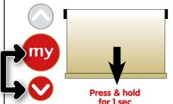
**4.3** To stop the blind at the desired lower limit position briefly press the **my** button (adjust with Up or Down if required).
