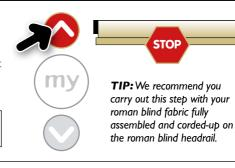
**4.2** Press and hold the **my** and DOWN buttons together until the blind starts to automatically move down (it will run until you complete the next step – so be prepared to stop at desired lower position).
