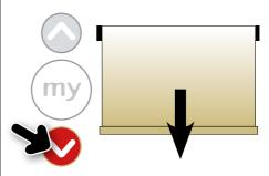
**TIP:** The motor is quick — so use short presses of the DOWN or UP button for accurate control.
