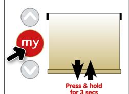
**3.2** Press and hold the DOWN button to test that the motor direction is correct.
