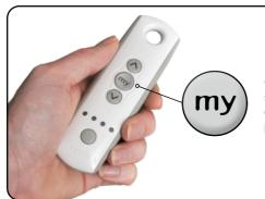
Once programmed, your remote will automatically stop at the set upper and lower limits when you press either the up or down buttons respectively, unless you press the **my** button, which will stop the blind.
